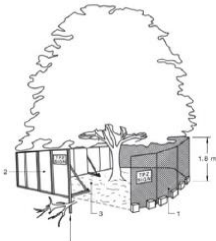
Example of TPZ fence from AS4970-2009 "Protection of Trees on Development Sites"
