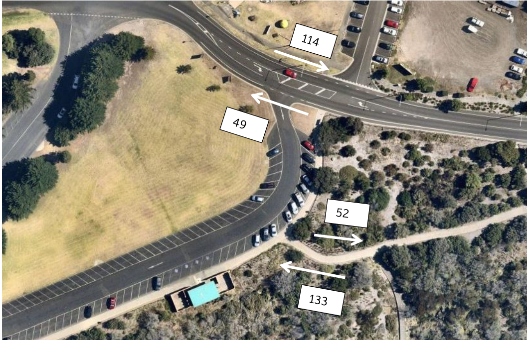
FIGURE 16: PEDESTRIAN COUNTS NEAR FERRY TERMINAL – SAT 6 FEB 10AM – 2PM
