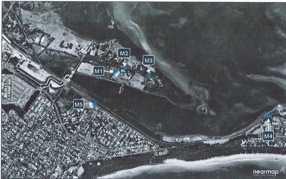
Figure 3 - Helicopter noise monitoring/measurement positions (source: Nearmap)
