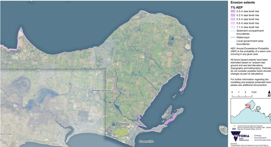
Figure 13. Erosion extent 1% AEP 2100 0.8m sea level rise
